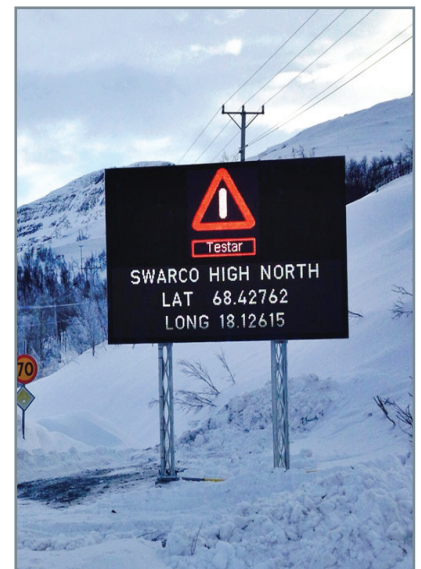
Free programmable variable message sign, full graphics, RGB Sweden
