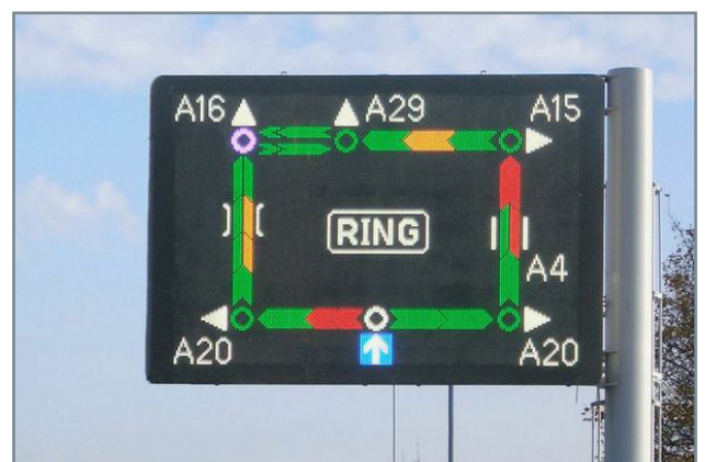
Free programmable variable message sign, full graphics, RGB, 16 mm pixel pitch
