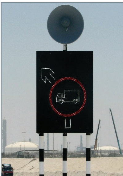
Limited variable message sign, dual color, integrated flashers United Arab Emirates
