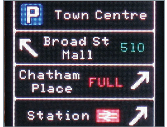
Free programmable parking guidance display, full color RGB, 16 mm pixel pitch United Kingdom
