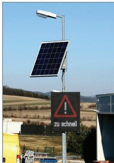
Radar activated/limited variable message sign powered by a PV panel Austria
